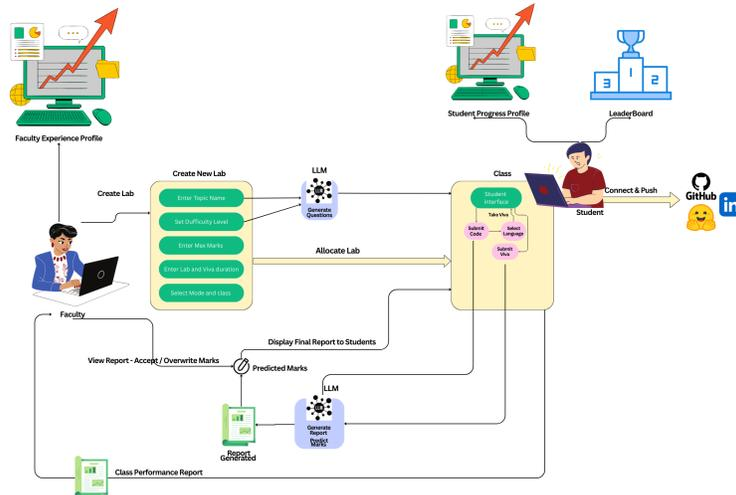
Figure 5: Detailed working Architecture of Ai-Lab Management Systems.
