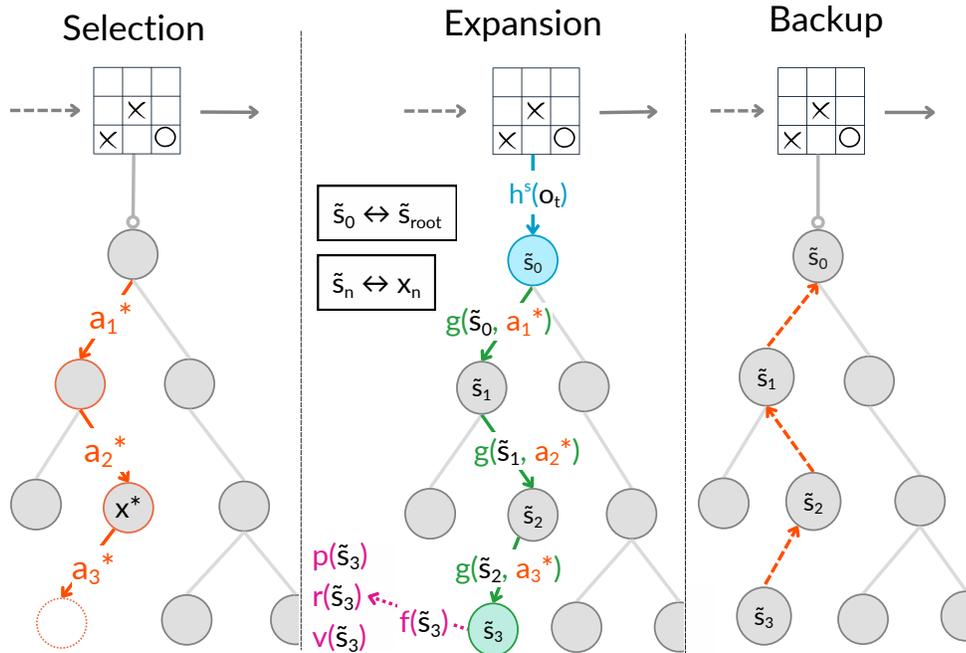
Fig. 1: MuZero’s MCTS process in latent space, showing selection using PUCT, expansion through the learned dynamics, and value backup to ancestor nodes.
